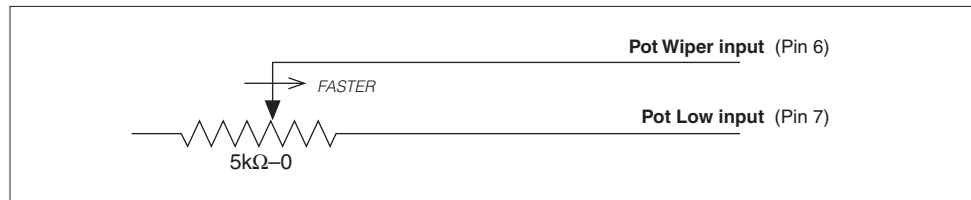
Fig. 4 Wiring for 5k \Omega -0 throttle (“Type 1”).
